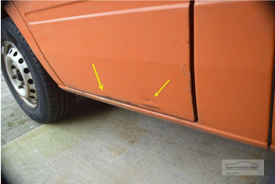
Rost Tür vorne links
