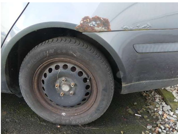
Rost hinten links
